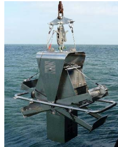
Small grab sampler Limited applications: highly disturbed sampled. Ok for PSA and basic seabed info.
