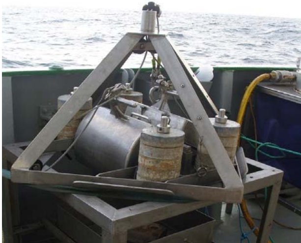
Small grab sampler Limited applications: highly disturbed sampled. Ok for PSA and basic seabed info.
