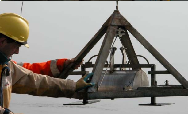
Box corer sampler Multiple applications: minimal disturbance. Good for PSA, sub surface geology, biological, chemical, geochemical. E-DNA, micro plastic, pollution monitoring.
