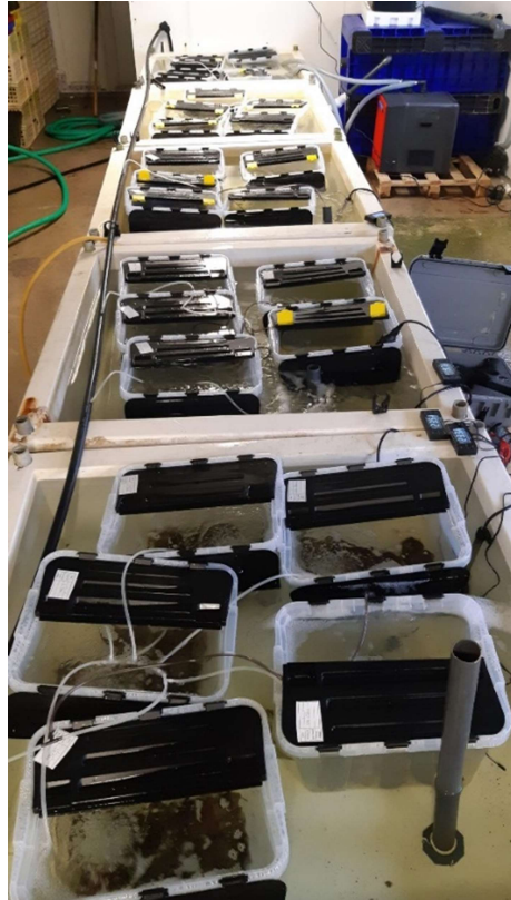
Figure 50. Experimental set up for assessment of response of oysters to 5 temperatures and 5 salinities (25 units). The temperature in each main container is constant and controlled by a combination of heating and chilling (essentially a water bath). There are 5 smaller containers at each temperature each at a different salinity. Aeration is provided by airstones.
