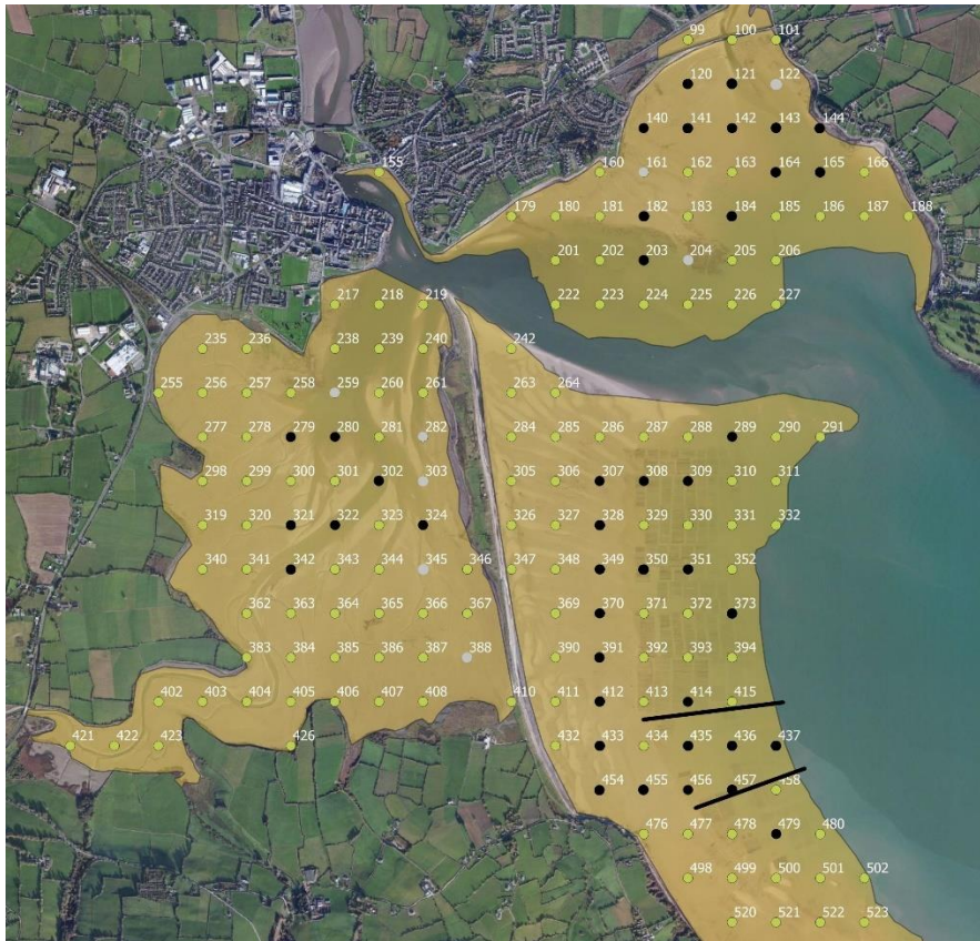
Figure 3. Sediment sampling grid with sediment sampling points shown in black (mostly sandy) or grey (mostly sand but with muddier components) where cores were taken in October 2020. The black lines show the approximate location of the (trestle-free) bird corridor. The list of sampled points is shown in Appendix 1.
